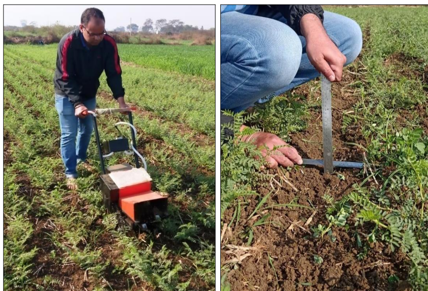
Fig 2: Field performance of battery operated single row weeder
