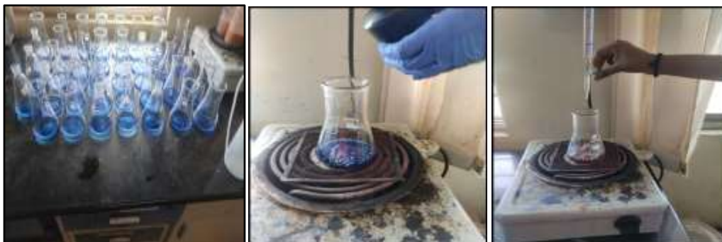
Fig 1: Total Soluble Sugar estimation – blue color turns to copper red on addition of sample through titration thus estimating total sugar amount in the sample
