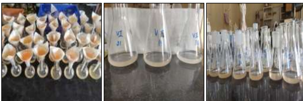
Fig 3: Estimation of Ascorbic acid- color turns to light pink color on addition of 2, 6-dichlorophenol indophenol dye
