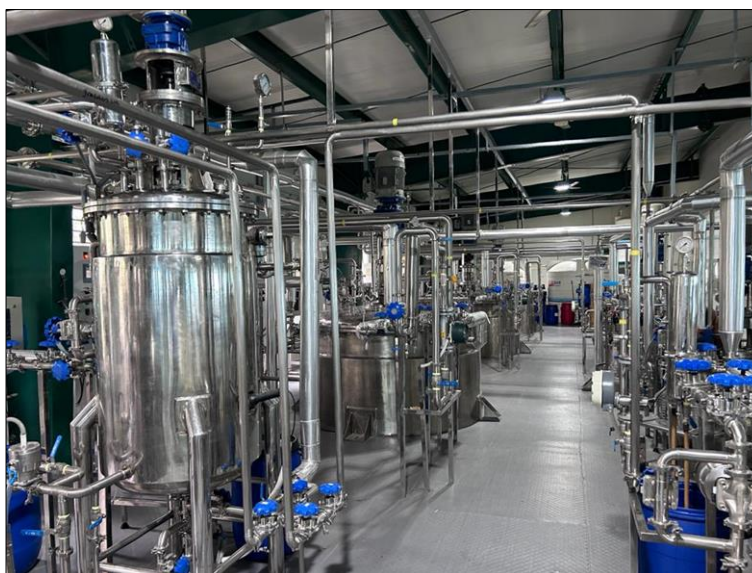
Fig 5: Commercial scale Mass Multiplication of Trichoderma in liquid state fermenter (Fermenter Capacity – 200 Lt to 5000 Lt)
