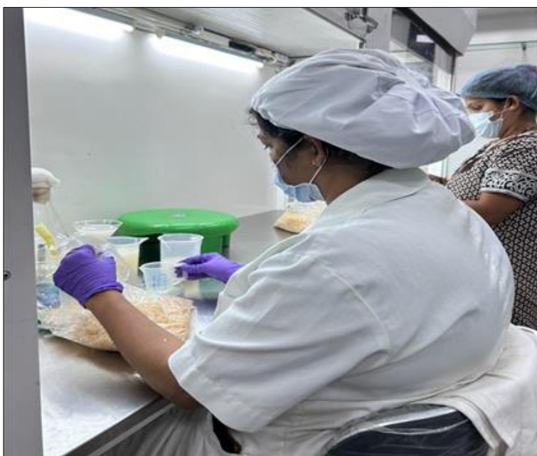
Fig 3: Microbial culture work performed under the biological safety cabinet and with specialized personal protective equipment (PPE).
