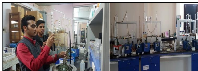
Fig 3: Distillation of lemongrass oil by Clevenger apparatus
