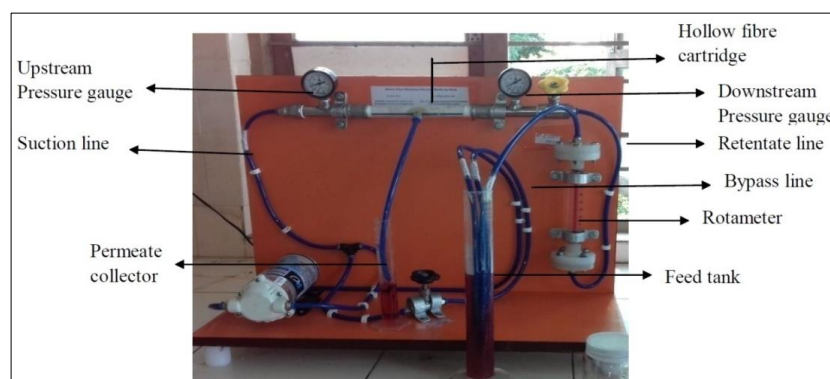
Fig 1: Hollow fibre membrane setup
