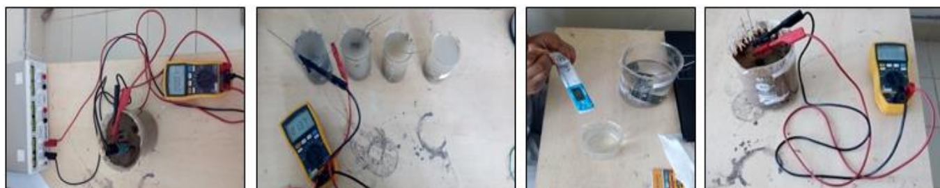
Fig 3: Electrode set-up and calibration for concentration measurement of NPK
