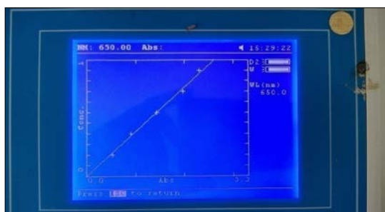
D. Prepare standard curve using by Spectrophotometer
