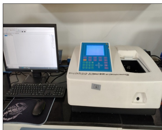
F. Measured on spectrophotometer at 645 and 663 wavelength
