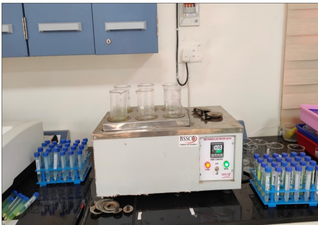
C. Evaporate standard by boiling water exactly for one minute
