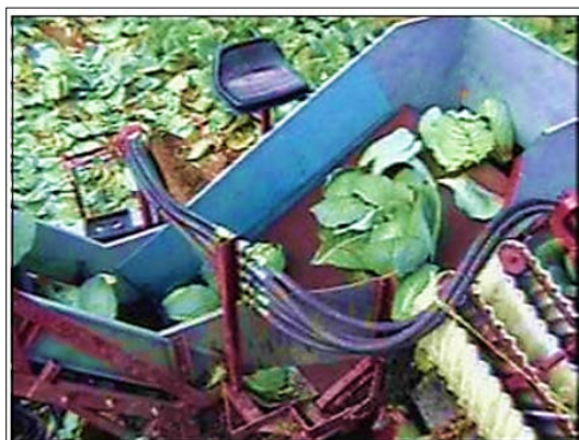
Fig 17: Prototype of the leaf separator (Chagnon et al. (2004) [6] )
