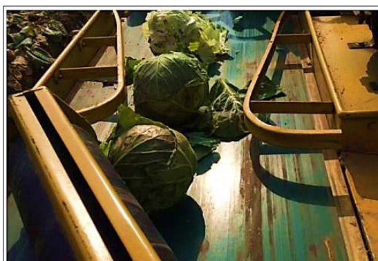
Fig 18: Leaf separator (Du et al. (2016) [13] )
