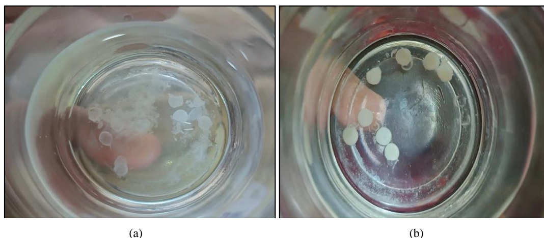
Fig 6: Bead stability in phosphate buffer: (a) beads that burst after 1 h; (b) beads that remained intact after 1 h
