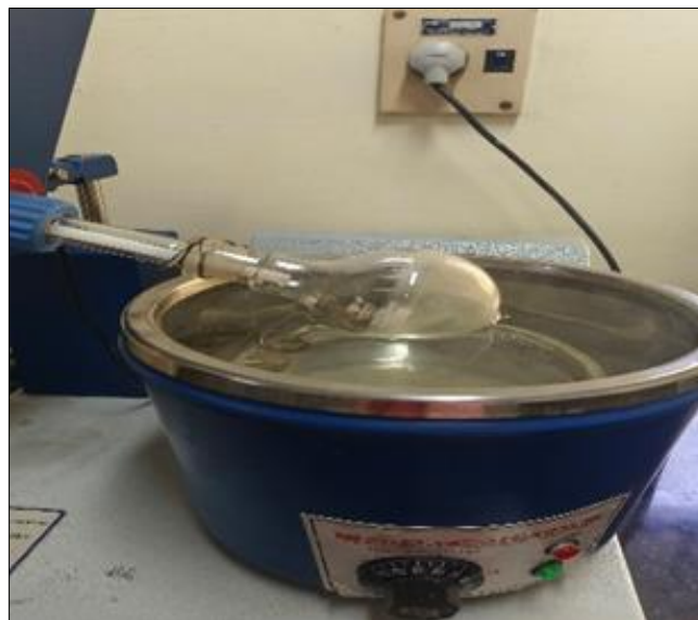
Fig 1: Thin film formation by rotary evaporator
