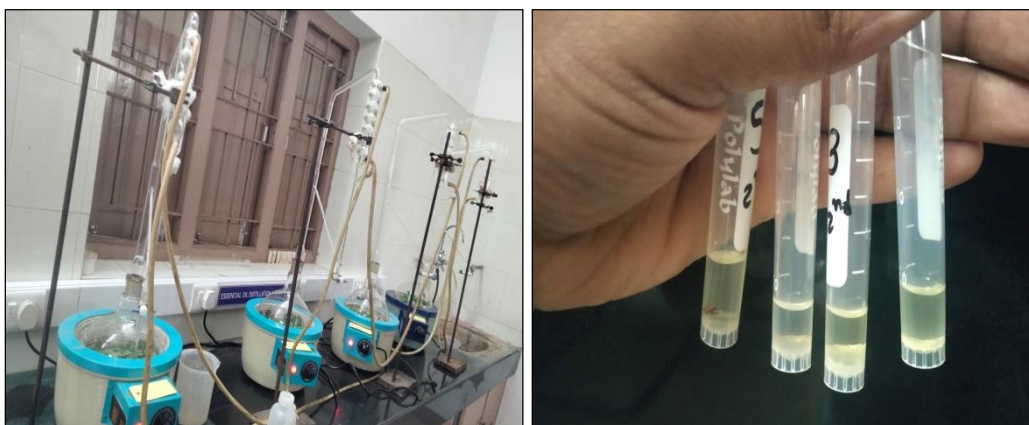
Fig 3: Hydro Distillation Unit and Leaf Essential oil of Sweet Basil
