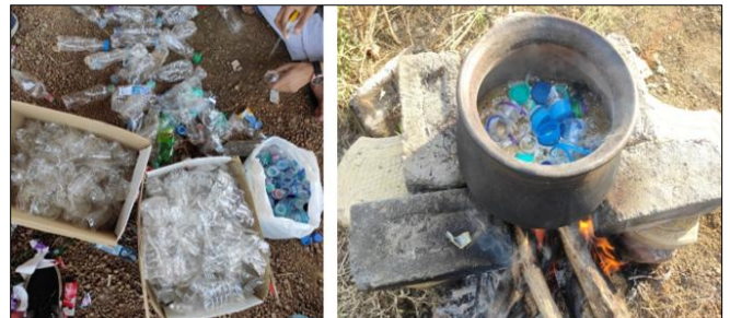
Fig 2.5 Showing cutting and melting of plastic.
