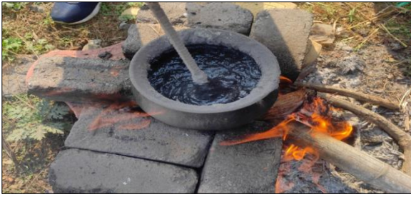
Fig 2.7: Showing mixing of fly ash and sand in melted plastic.
