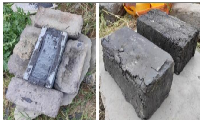
Fig 2.6: Showing the Moulding and de-moulding process
