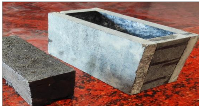
Fig 2: Showing making of bricks mould by using granite.
