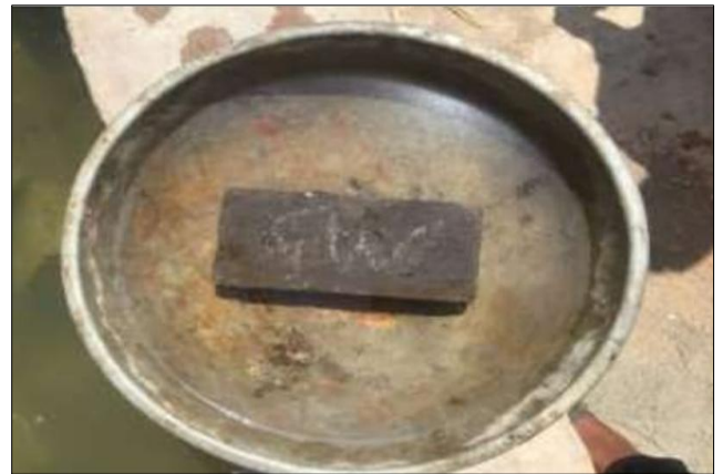
Fig 3.2: Water absorption tests of plastic bricks
