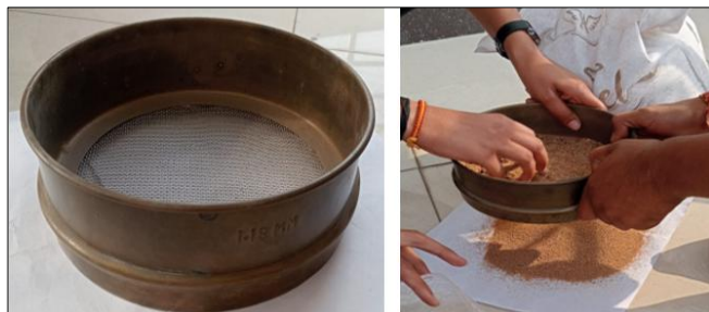
Fig 2.3: Showing sieve and sieving of sand
