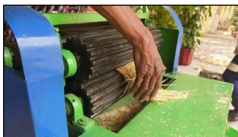
Fig 4: Operational view of the power-operated linseed fiber extraction machine during fiber extraction process.
