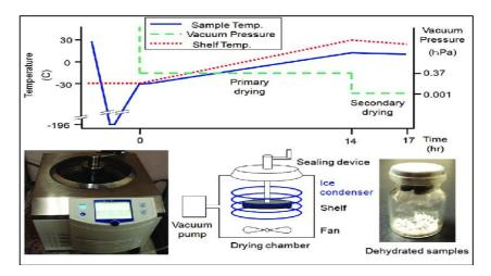
Kinetics of Vacuum Pressure and Shelf Temperature Programmed for a SpermFreeze-drying Protocol in a Freeze-dryer Machine (ALPHA 2-4 LSC) (Hochi *et al.*, 2011) [15].
