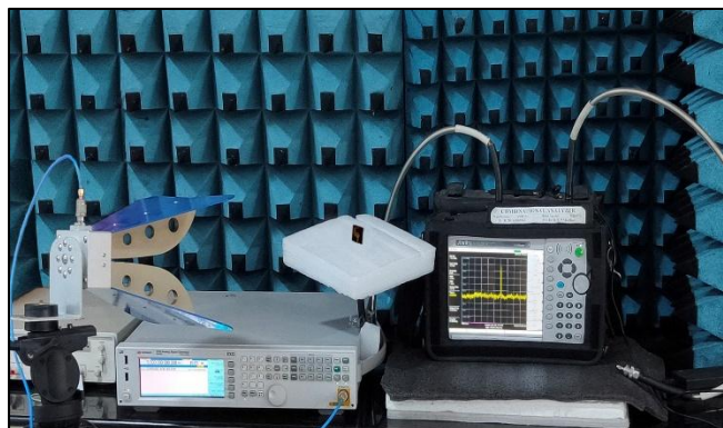
Fig 7: Measurement setup of the in vitro blood absorbed antenna for measuring the 5.8 GHz test signal.
