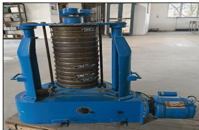
Fig 4: Measurement of fineness modulus size using sieve shaker
