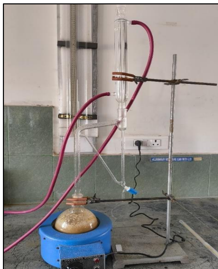
Fig 3: Clevenger's apparatus for volatile oil extraction.
