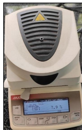
Fig 1: Moisture measurement using Axis ATS moisture meter
