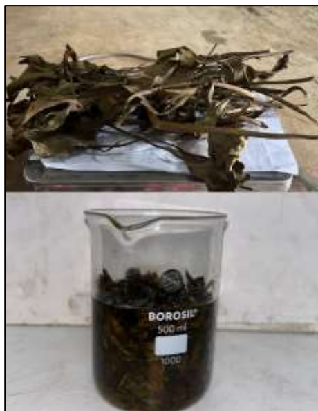
Fig 4: Delignification of Water hyacinth after drying
