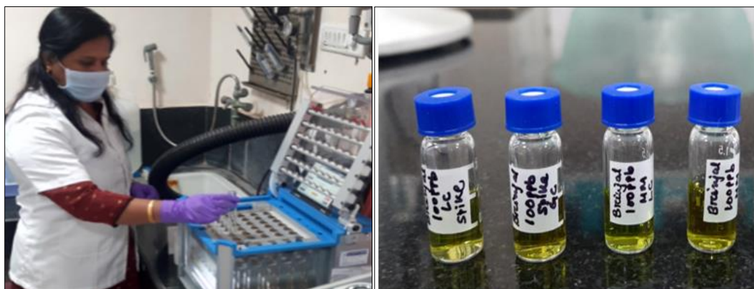
Fig 12: Evaporating to dryness using nitrogen concentrator Fig 13: Final 1.5 ml extract into LC auto sampler vials
