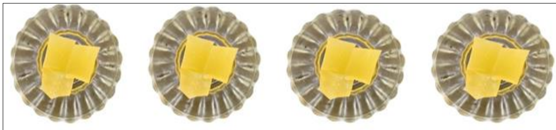
Fig 5: 5 (A), Fig 5(B), Fig 5(C) and Fig 5(D) represents carrageenan gels kept at 20 °C, 25 °C, 30 °C and 35 °C. From the figure, it is clear that gels were stable even at a higher temperature of 35 °C.
