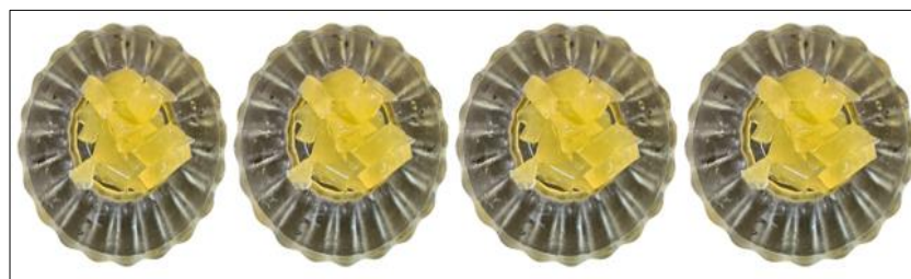
Fig: 4(B), 4(C) and 4(D) represents agar agar gels kept at 20 °C, 25 °C, 30 °C and 35 °C. They were stable even at a higher temperature of 35 °C.
