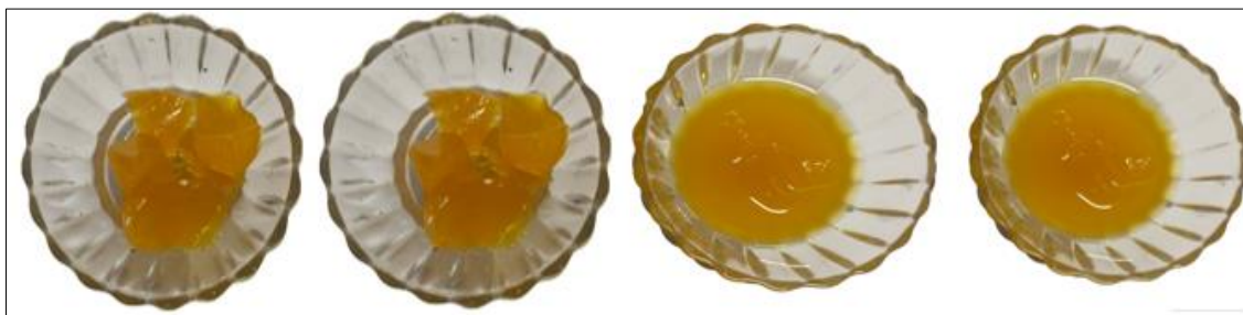
Fig 6: 6(A) and 6(B) show that gelatine gels remained stable at 20 °C and 25 °C whereas Figure 6(C) and 6(D) reveals that gelatine gels melted at temperatures 30 °C and 35 °C respectively
