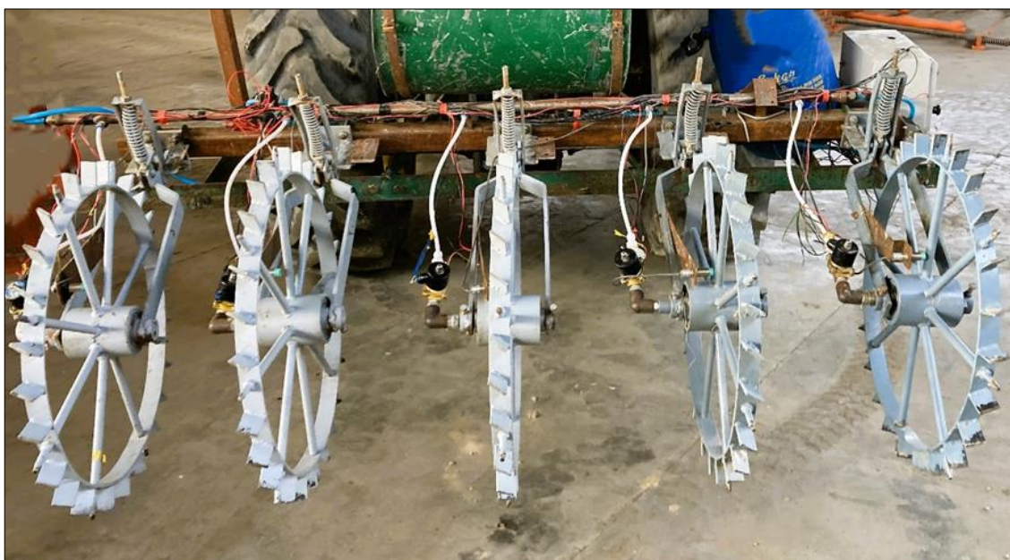
Fig 3: Real view of spoke wheel type liquid urea applicator
